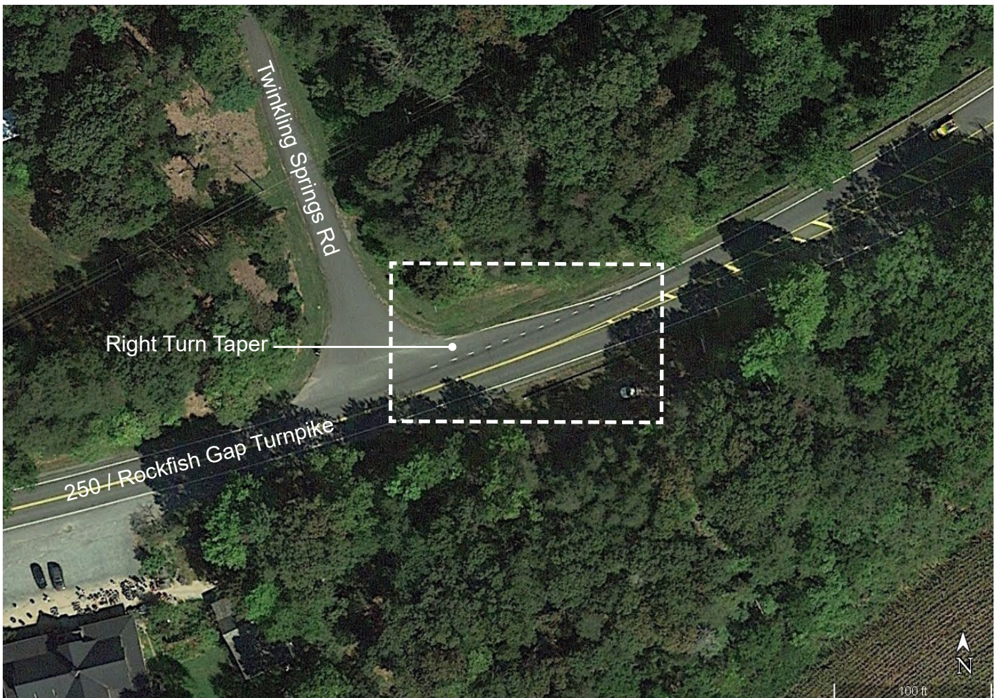
Figure 4 – Existing Right Turn Lane
